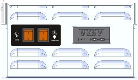
2. Set the temperature control to the desired temperature setpoint by pressing the set button on the controller. Use the up or down arrows to raise and lower the temperature setpoint. Once the desired setpoint is entered, press the set button one more time to save the setting.
