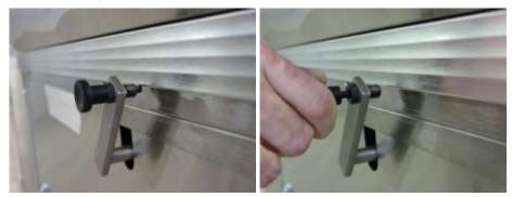
3. If equipped with the motorized option, the bin level is adjusted by pressing down on the elevator switch to lower and up to raise.
