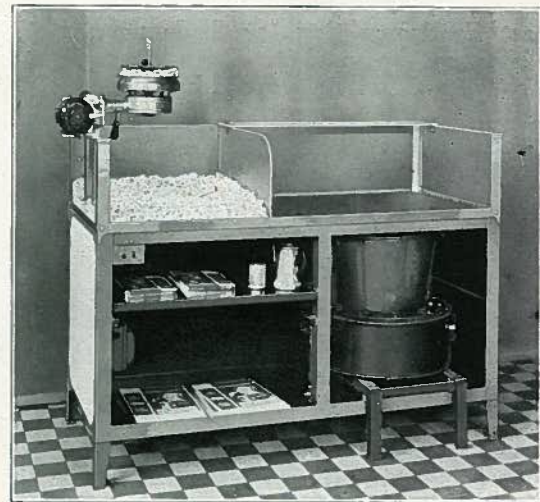
"PULL-OUT" CANDY FURNACE Showing how furnace and crisp kettle push into base of machine out of the way, when not in use. Removes furnace heat from work table when making crisp. (Patented.)
