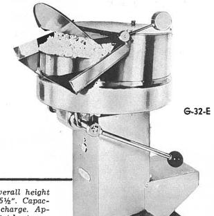
BASIC SPECIFICATIONS—Giant 32-oz. Electric Model: Overall height to top of pan 27". Stainless steel base measures 8" x 15½". Capacity: 2 lbs. of raw corn and 11-oz. of popping oil per charge. Approximately \$75.00 per hour. Fully automatic thermostat heat control. 115V/230V, 60 cycle, A.C., three-wire, single phase. Number 10 or larger wire necessary with direct feed. Total Wattage: 4700.
