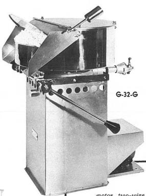
BASIC SPECIFICATIONS - Giant 18-oz. Electric Model: Overall height to top of pan 27". Stainless steel base measures 8" x 151/2". Capacity: 18-oz. of raw corn and 6-oz. of popping oil per charge. Approximately \$50.00 per hour. Fully automatic thermostat heat control. Standard 115/ 230 volt, 60 cycle, 3 wire service. (is available 115 volt, 60 cycle, 2 wire service as special order.) Number 10 or larger wire necessary with direct feed. Total Wattage: 2700.
