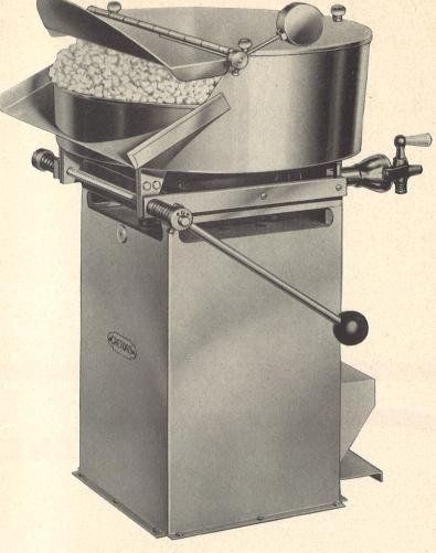
height to top of pan: 26". Stainless steel base measures 11¼" x 17½". Capacity: 2 lbs. of raw corn per popping, \$75.00 per hour. 110V. 60-cycle agitator motor. Enclosed transmission. Burns Natural, Manufactured, or Bottle Gas (specify which when ordering). Gasoline equipment optional at extra cost. Shipping weight: 85 lbs.
