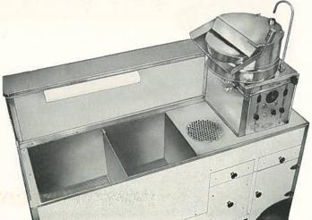
**CUTAWAY ILLUSTRATION** shows the tremendous amount of storage capacity in the stainless steel storage bin. Note the movable divider which allows storage of varying amounts of boxed and popped corn. Quality of the stored corn is maintained and protected by the Exclusive Cretors CORNDITIONER.
