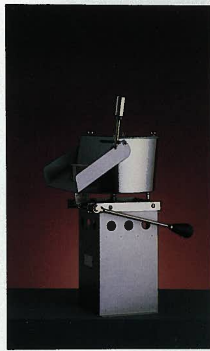
Model G12G Little Giant 12 Gas Popper CAPACITY: 12 Oz. All-Steel Kettle—285 one-ounce servings per hour ELECTRICAL: 120 Volt, 60 Cycle, Single Phase, 2 Wire, 100 Watts, 1 Amp (Opt. 12 Volt D.C. available) SPECIFY NATURAL OR BOTTLED GAS. DIMENSIONS: Base: 6½" x 7½"; 23" T NET WEIGHT: 20 lbs. Shipping Weight: 26 lbs. SHPG. CARTON: 14½" D x 14½" W x 25" T; Cube: 3
