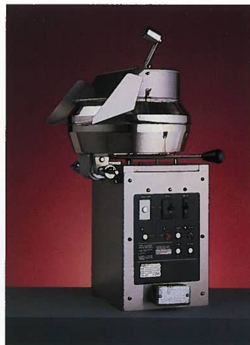
Model G20E Giant 20 Electric Popper CAPACITY: 20 Oz. All-Steel Kettle 400 one-ounce servings per hour ELECTRICAL: 120/208 or 120/240 Volts, 60 cycle, Single Phase, 3 Wire, 2950 Watts, 14 Amps DIMENSIONS: Base: 10 1/2" x 31" T NET WEIGHT: 63 lbs. Shipping Weight: 75 lbs. SHPG. CARTON: 22" D x 25" W x 35" T; Cube 11
