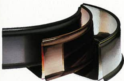
The three layers of Cretors exclusive plating process are shown here. From left to right, there is the raw steel which has been cleaned and pickled, the copper which is flashplated to the steel and lastly an extra-heavy layer of nickel which is plated to the copper and then meticulously cleaned and polished.
