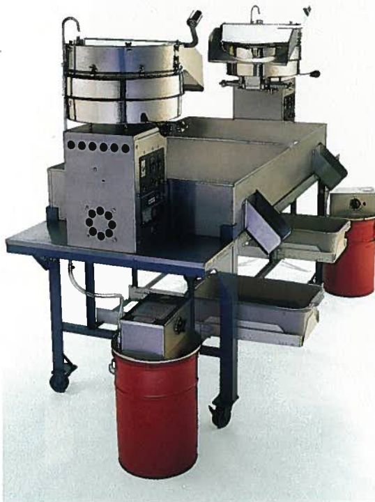
Model TGS32EP Twin Giant Special Electric with Pump CAPACITY: 2-32 Oz. All-Steel Kettles-640-one-ounce servings per hour per popper. ELECTRICAL: 120/208 or 120/240 Volts, 60 cycle, Single Phase, 3-Wire, 5250 Watts, 28 Amps per popper DIMENSIONS: Frame: 79" D x 30" W x 61" T Pan: 57" D x 30" W x 8" T NET WEIGHT: 386 lbs. Shipping Weight: 540 lbs. SHPG. CARTON: 89" L x 41" W x 68" T; Cube 143.5
