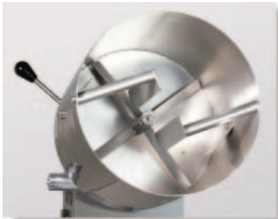
Cretors exclusive mixing baffles shown on CMD 25
