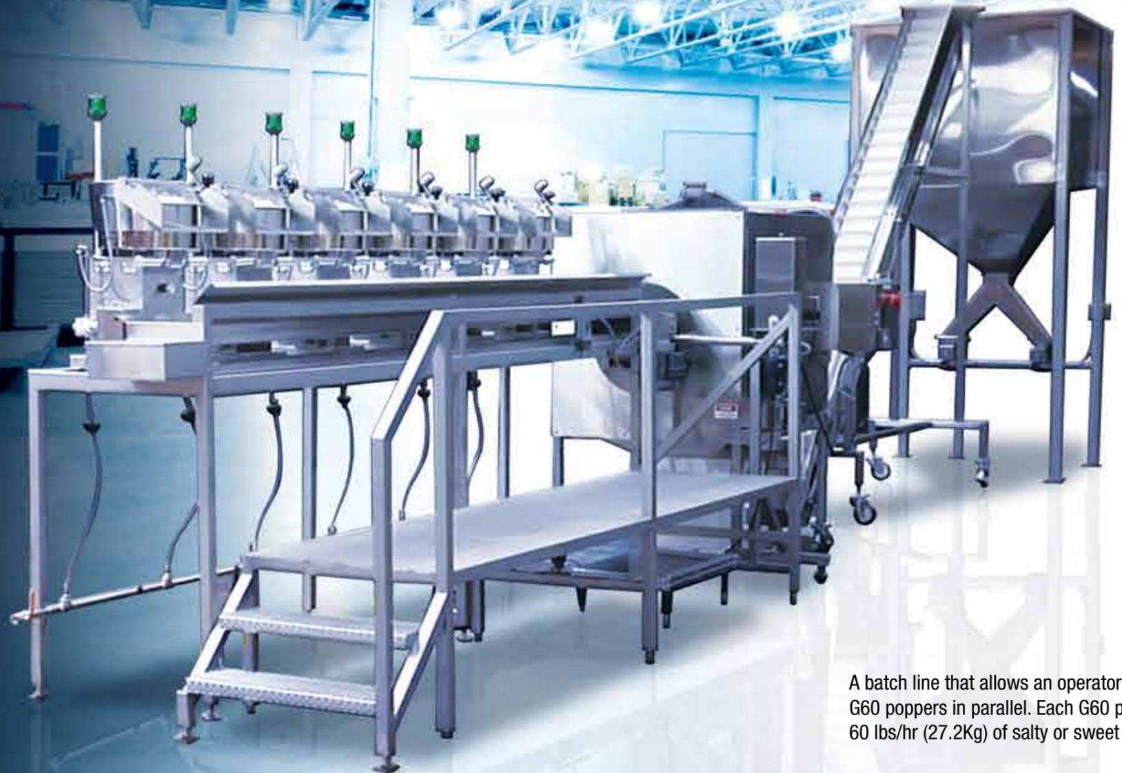
A batch line that allows an operator to run a number of our G60 poppers in parallel. Each G60 popper can produce up to 60 lbs/hr (27.2Kg) of salty or sweet popcorn.
