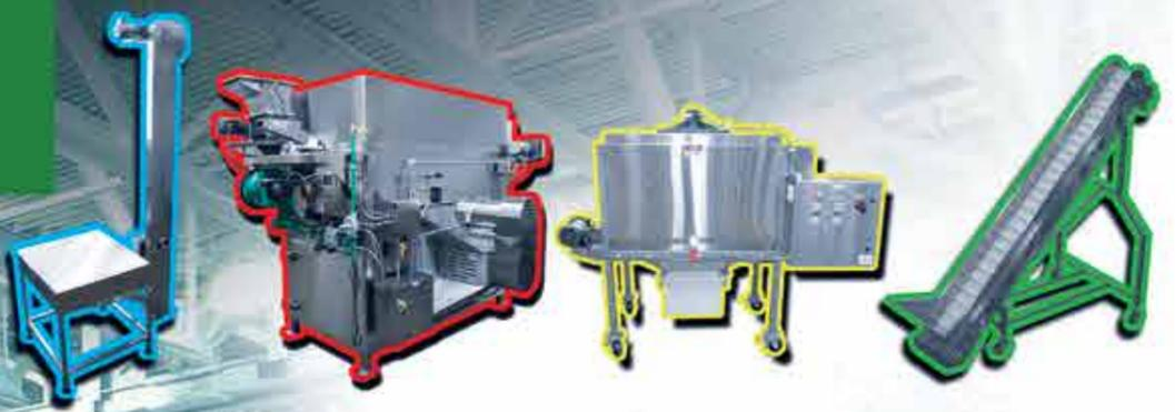
A single Kettle /Coater line that will typically produce 350lbs/hr (160Kg/hr) of Caramel Corn. A twin Kettle/Coater line will produce double that.
