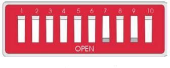
Switch #6 = 5 seconds #7 = 10 seconds #8 = 20 seconds #9 = 40 seconds
