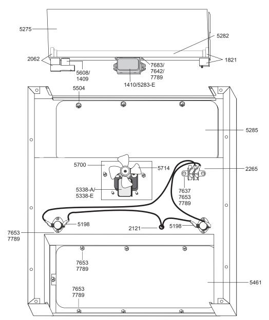
1410 BALLAST 20 WATT 1821 SOCKET-FLUORESCENT LAMP HOLDER-COMB. 2062 2121 BUSHING **TERMINAL BLOCK** 2265 THERMOSTAT 5198 5275 LIGHT REFLECTOR 5282 LAMP-FLUORESCENT 5285 PLEXIGLASS LIGHT COVER 5283-E **BALLAST 230V** 5338-A **BLOWER MOTOR** 5338-E **BLOWER MOTOR** 5461 LIGHT COVER 5504 8-32 HX SERRATED FLANGE NUT
